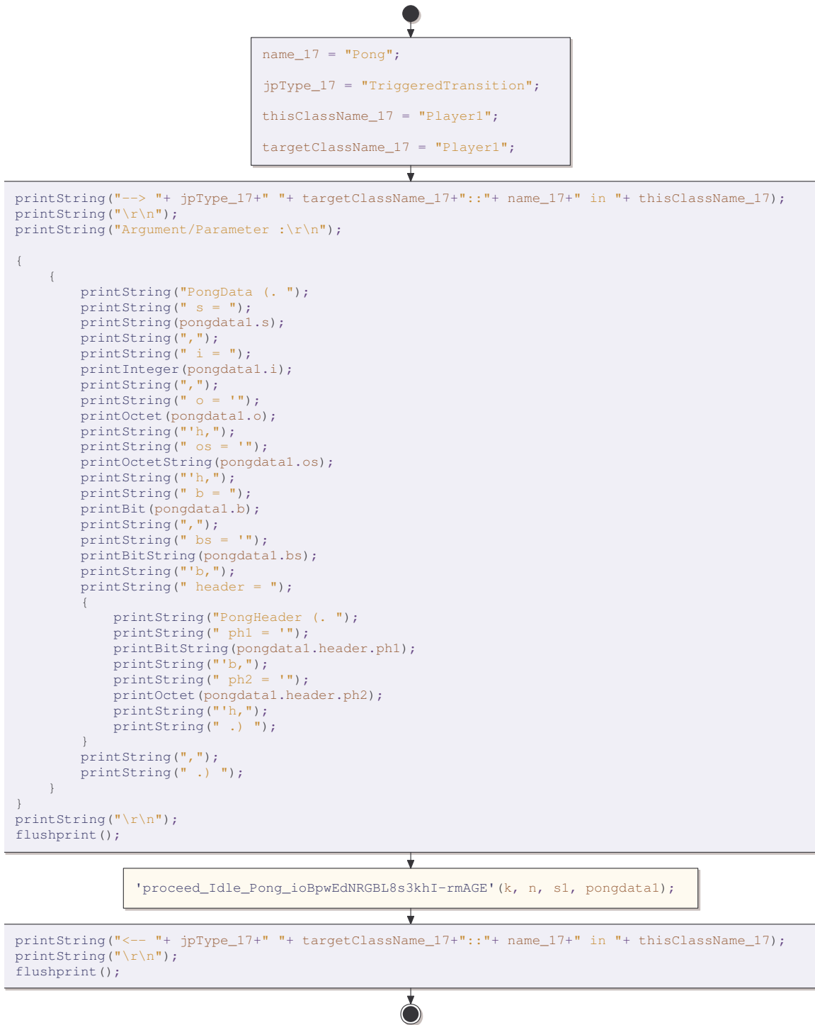
Figure 12. Connector Instance in the context of class Player1, as displayed when clicking on the input symbol corresponding to the Pong triggered transition
