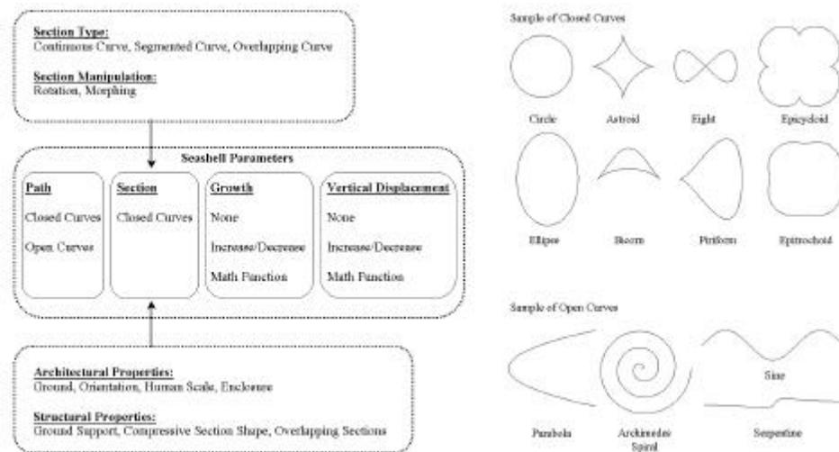
Figure 2. Architectural form generating diagram and mathematical curves
