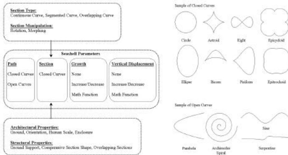
**Figure 3. Architectural form generating diagram and mathematical curves.**
