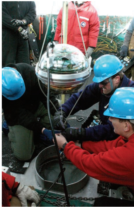
Brrr! Researchers constructing Ice Cube lower a photodetector into the South Pole ice.
